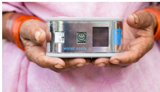
Figure 1 Wadi for water purification via solar energy, developed by Helioz ( https://www.trendingtopics.at/wadi-who/ )
